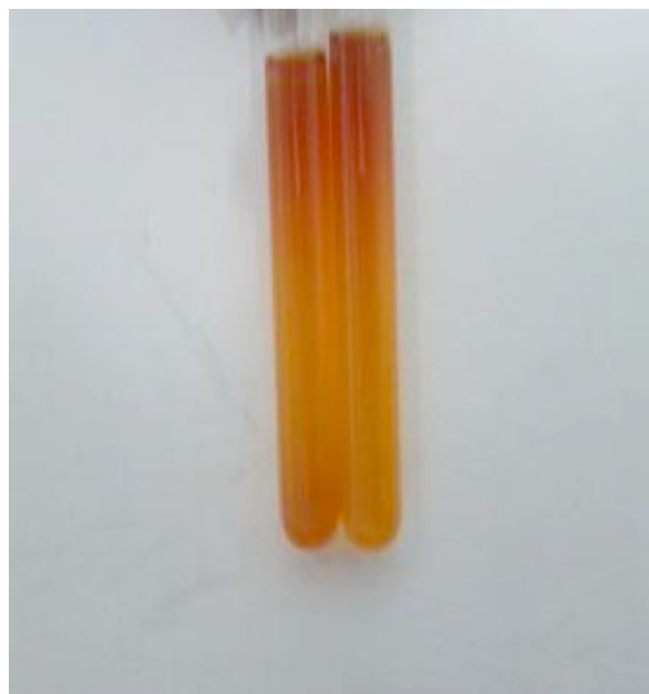
Figure 2: FAX gels irradiated with 6 MeV electrons. With decrease in absorbed dose from top to bottom of the cuvettes, the color intensity of gels becomes lighter.
