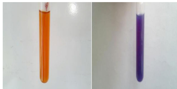
Figure 1: FAX gel before (orange) and after irradiation (purple) by 9 MV photon beam
