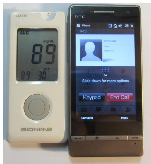
Figure 1: Position of the mobile phone and the BIONIME home blood glucose monitor during measurement.
