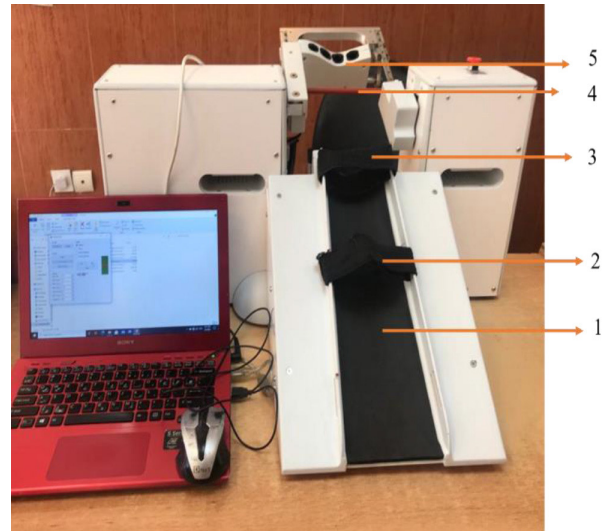
Figure 6: The setup of the test, 1) hand stand, 2) bottom strap, 3) top strap, 4) elastic cable, and 5) fingers cover
