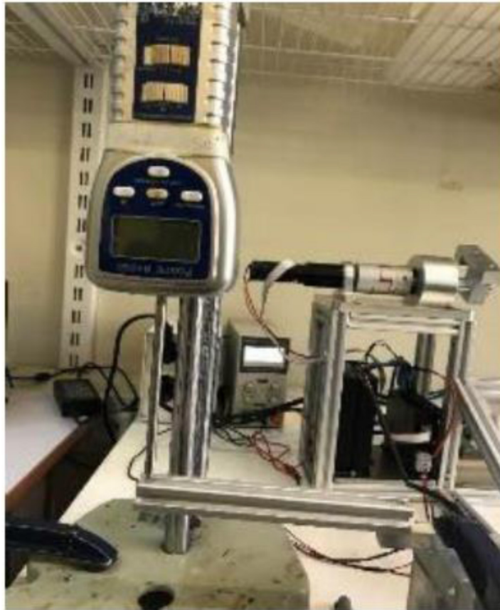
Figure 3: Loadcell calibration in force-gauge
