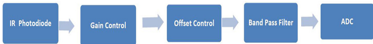
Figure 3: The light detector circuit includes steps of detecting, amplifying, removing noise, and finally converting the optical signal into a digital signal.
