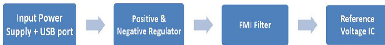
Figure 1: Block diagram of the power supply circuit of the designed non-invasive blood glucometer.
