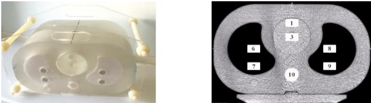
Figure 2: Cirs-like phantom properties: soft-tissue: PMMA bone: tetraflouroethylenteflon lung: Cork Long: 21cm width: 35cm height: 20cm slice thickness: 9mm
