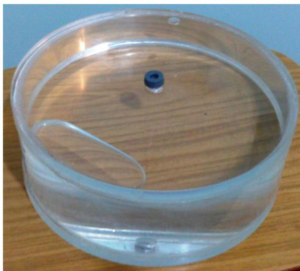
**Figure 1:** Home-made acrylic cylindrical MRS quality control phantom which contains the metabolites mimicking the brain metabolite combination.
