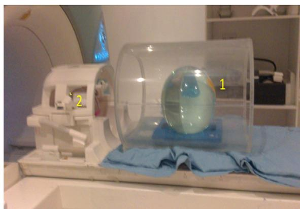
**Figure 2:** The position of phantoms for QA test. 1- body loader phantom. 2- spherical QA phantom inside the head coil.
