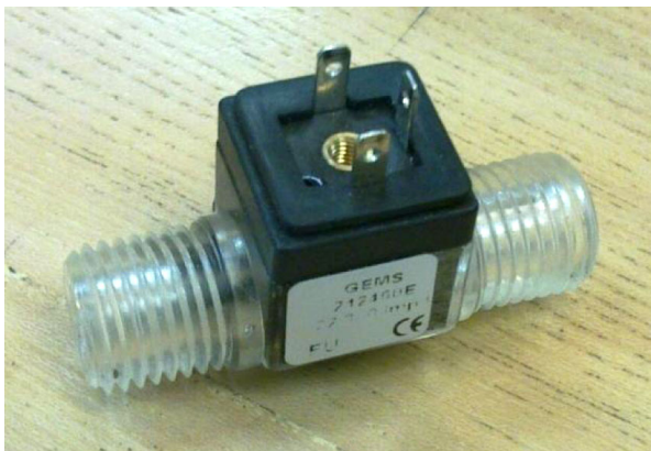
Figure 2: The flowmeter: The three pins are for power supply, ground and output signal
