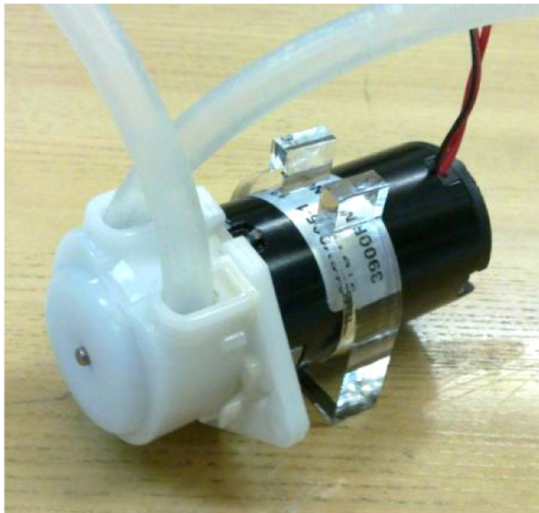
Figure 1: Peristaltic pump used for both injection and drainage of the dialysate
