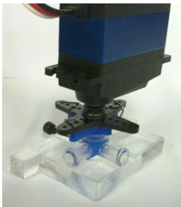
Figure 3: Triway valve with attached servomotor
