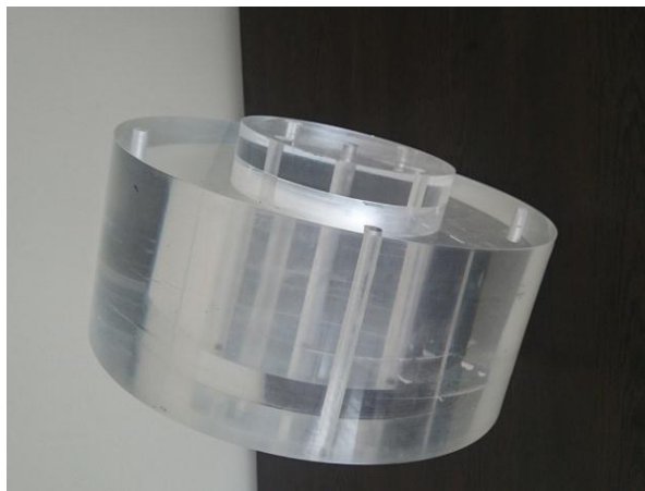
Figure 1: Head and body CT dosimetry phantom
