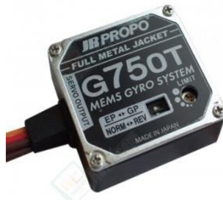
Figure 4: G750T MEMS Gyro System
