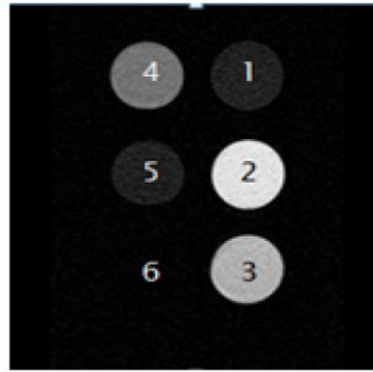
Figure 1: Coronal image of the phantom containing test tubes with different contrast concentrations. Positions of different doses of the contrast agent are determined in this image with numbers and other images in this paper have the same position.
