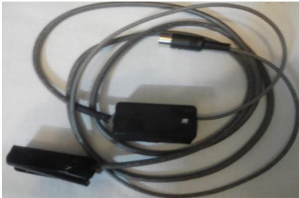
**Figure 1:** PPG probe designed in this project for recording in four wavelengths
