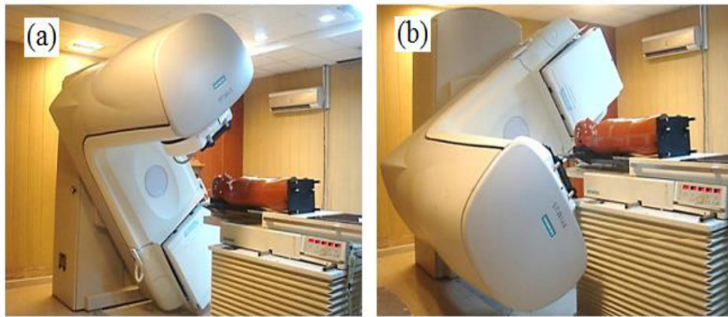
Figure 3: Irradiation setup of the RANDO phantom with right anterior-oblique (a) and right posterior-oblique (b) fields in measurement of skin dose in radiotherapy of parotid cancer.
