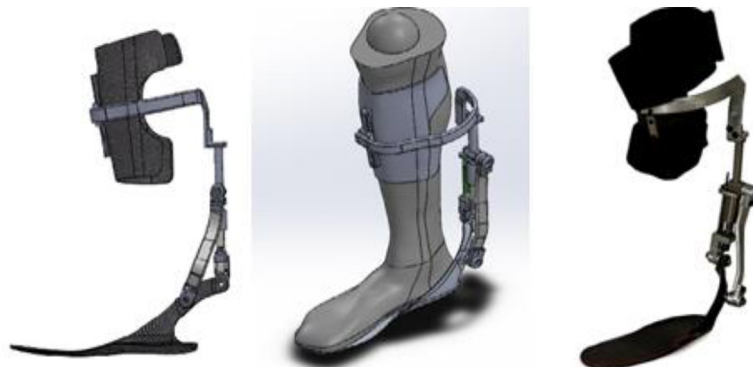
Figure 1: Novel hybrid passive spring damper ankle foot orthosis
