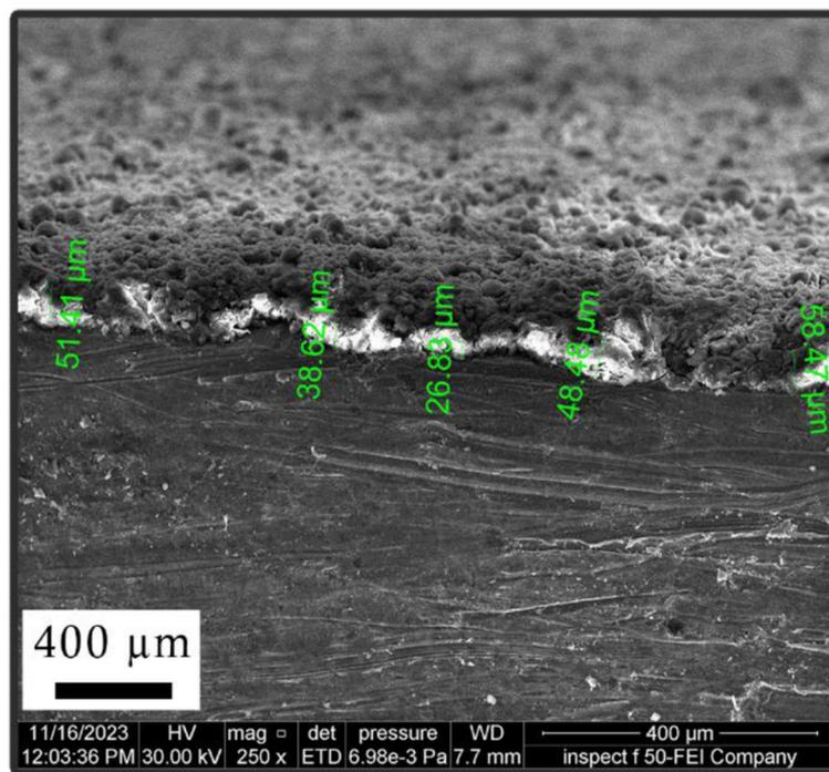
**Figure 5:** Cross section for the coated disc.
