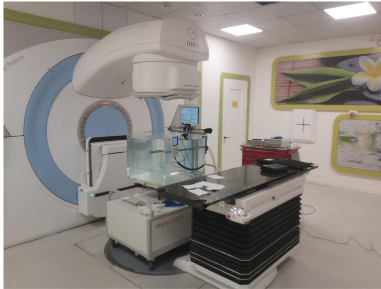
Figure 2: Absolute dosimetry was conducted using a linac (Elekta Synergy Platform) in conjunction with a Pole To Win (PTW) Motorized 3D water Phantom system (MP3) to measure the effective wedge angles.
