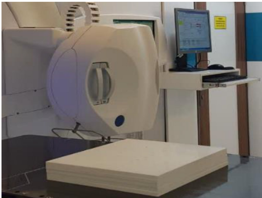
Figure 2: The necessary slab (PTW (Physikalisch-Technische Werkstätten), Germany) thickness (2 cm for 6 MV & 3 cm for 10, 18 MV) for build-up conditions was placed on the Thermoluminescent Dosimeters (TLDs), depending on the energy level
