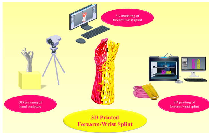
Figure 3: Schematic workflow of the personalized 3D-printed forearm/wrist splint fabrication process
